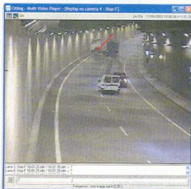
Automatic incident detection in operation in a tunnel
