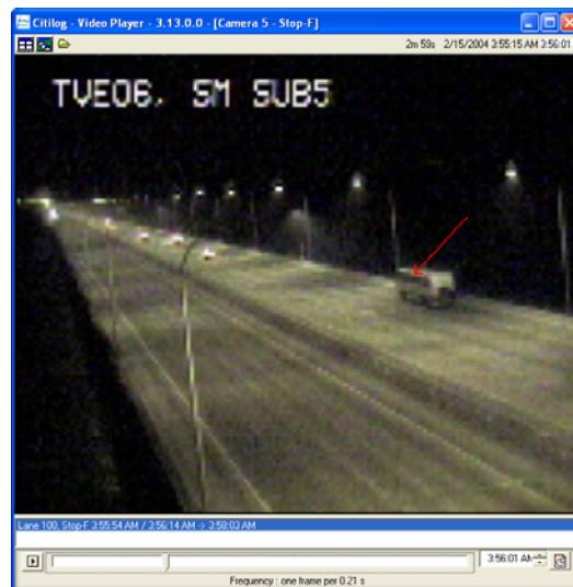
Figure 2 – Detection of a bus stopped at night on the San Mateo Bridge
